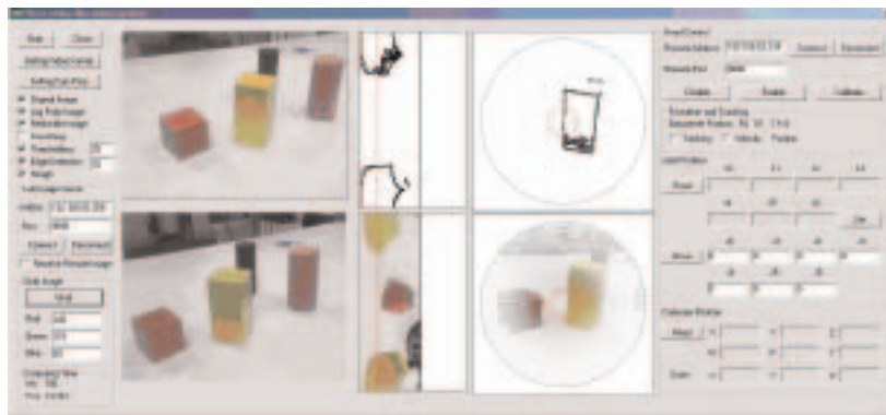
Figure 16. An example of a retina-like image with the corresponding log-polar projection and of a step of visual processing (edge detection).
