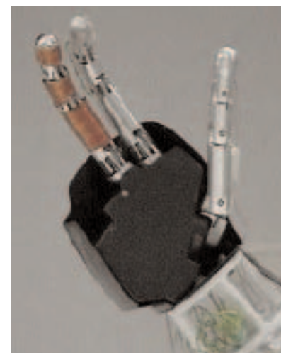
Figure 13. The three fingered Paloma hand. The thumb has 3 phalanges and a trapezometacarpal (TM) joint with 2 DOFs placed at the base of the palm, near the wrist, that allows the movement of the thumb along the flexion plane in order to allow several grasping configuration.
