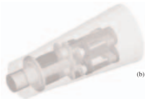
Figure 10. (a) The five fingered hand is underactuated: 16 Degrees of Freedom (DOFs) are actuated by six motors. Five ((b) integrated in the socket) control the fingers flexion and one (integrated in the palm) control the thumb abduction/adduction. The estimated grasping force is 45 N. The estimated total weight (including the actuation system) of the CYBERHAND biomechatronic hand is about 700 gr. and the dimensions are: 191 mm (total length), 92.2 mm (length of fingers), 14 mm (diameter of fingers), 95 mm (palm width), and 40 mm (palm thickness).
